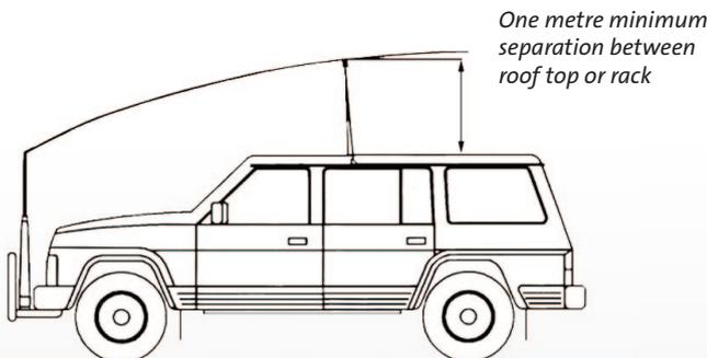
Antenna mounted at bumper bar height
