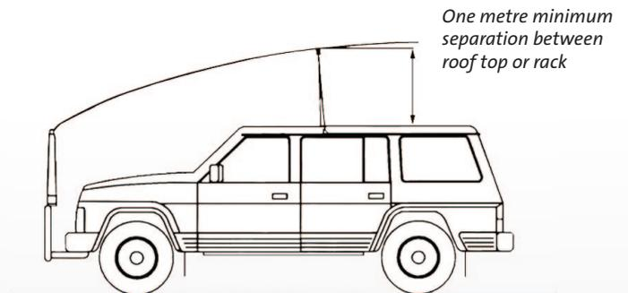
Antenna mounted on bull bar
